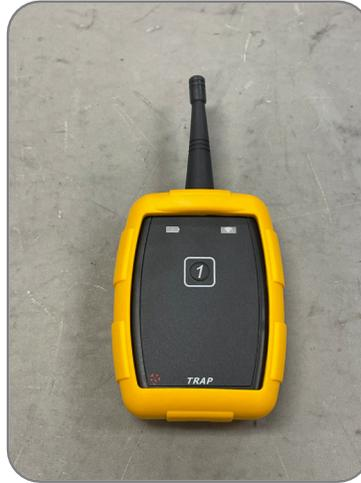
If you are receiving a negative acknowledgement on the transmitter (blinking red LED), try with better line of site or closer distance to the receiver. It is recommended to get a visual of the remote beacon systems to ensure they have been triggered instead of relying on the transmitter acknowledgement LED.
