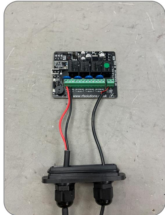
7. Connect the power cable to the barrel connector splitter temporarily. Connect the R838 AC/DC power supply to the splitter. Plug in the power supply to an available outlet to power up the receiver. You should see a red PWR LED on the circuit board showing the board has initialized.
