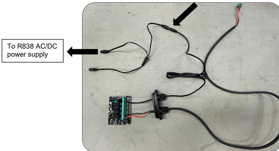
8. Locate the jumpers on the top of the circuit board. Place one of them on LK3. The circuit board will beep confirming you are in setup mode.
