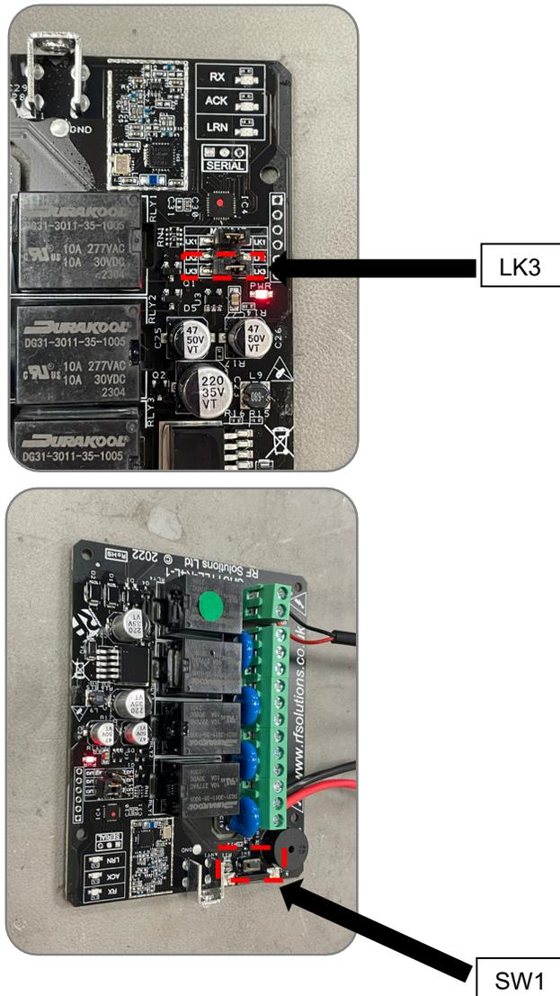
11. Reinstall receiver circuit board, antenna, and access panel. Ensure gasket is seated properly.
