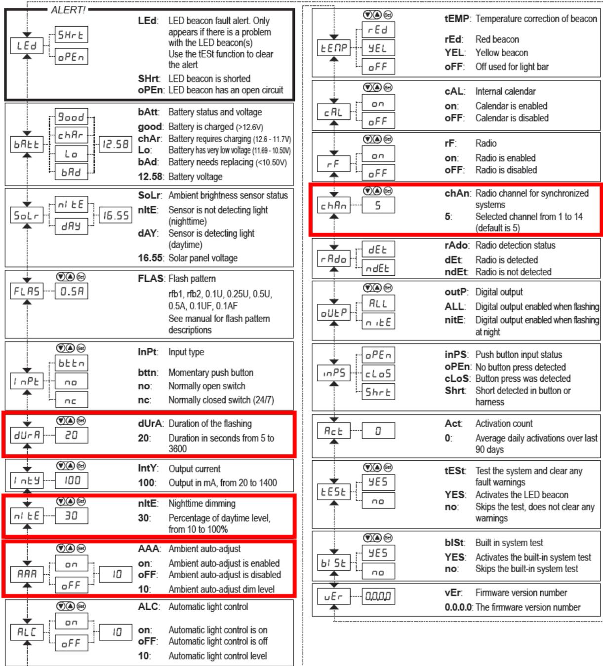
The following sections describe how to change the R838's Flashing Duration, Night Dimming, Ambient Auto-Adjust, and Radio Channel:
